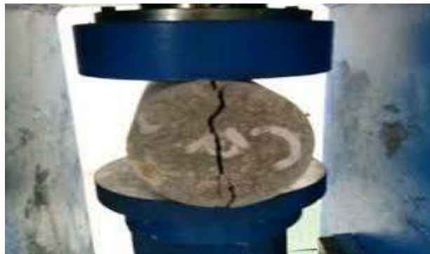
Fig 4.11.1.2 failure of cylindrical specimen in Split tensile test
